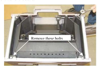
8. Use a ½" wrench to loosen the locking bolts located on the inside of the door frame. Release the lock nut then turn the bolt to relieve the tension against the front wall.
