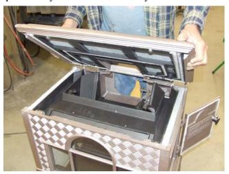
7. Use a ½" socket to remove the two bolts that hold the front of the combustor pan to the front wall of the stove.
